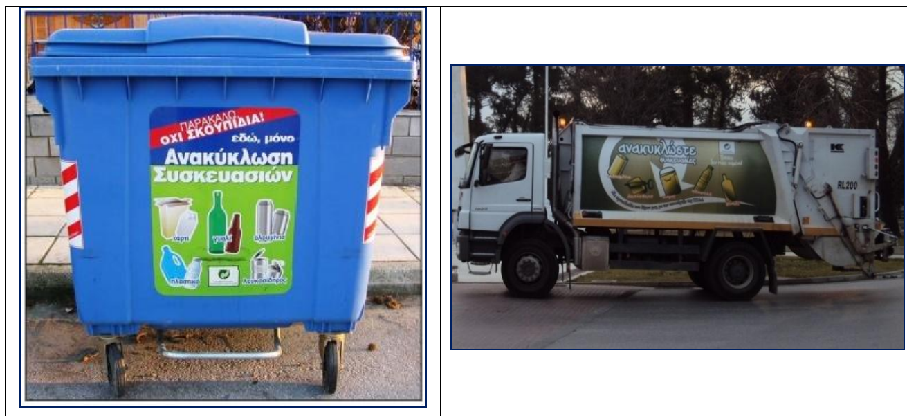
Picture 4. Recycling plastic blue bin of 1.100lt and refuse compression collector vehicle for packaging recycling.
