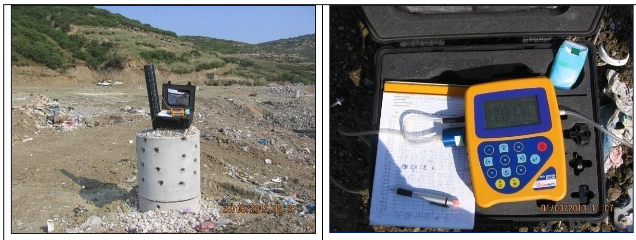
Picture 9: Photos of landfill gas recording in sanitary landfill in Kavala.
